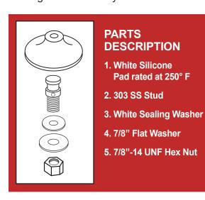
inside the lower cone of the bin along areas where material tends to stick or bridge. By combining both aeration and vibration, the Airbrator can resolve some of the more difficult material flow applications that aeration alone cannot.
