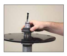
21. The neck nut is then installed on top of the mounting plate.
