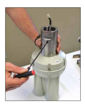
9. Then take the extension cable and hook it up so the locking mechanism connects, making sure the locking tab connects.
