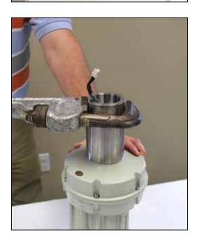
7. It simply screws onto the neck of the scanner. Snug the adapter to the transducer using a 24-inch pipe wrench.
