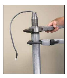
16. Once again, tighten using two 24" pipe wrenches, one backing up the pipe and the other tightening the adapter.
