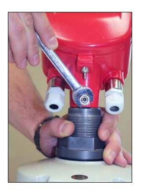
23. Tighten the hex set screw with a 5/32" allen wrench and secure the lock nut with a ½-inch wrench.
