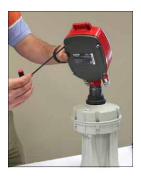
1. Start by removing the back plate from the electronic enclosure by undoing four screws with a 5/32" allen wrench.
