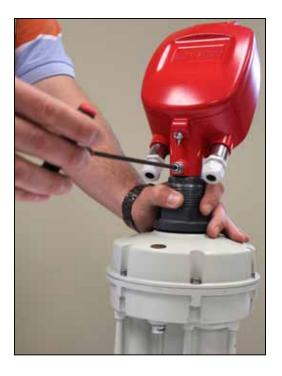
22. Next, the electronic enclosure is ready to go back on; it can be installed in 45 degree increments.
