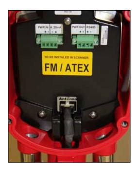
2. Inside the enclosure, you will disconnect the 10-pin connector from the electronic card and pull out the cable strain relief.
