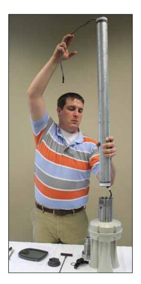
12. The next step is to fish the cable through the extension pipe.
