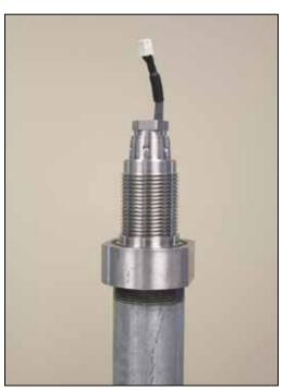
17. Insert the remaining cable into the pipe by twisting and pushing the cable down into the extension until there is about 3" of cable exposed.
