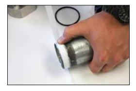
11. Prepare the extension pipe with about three wraps of Teflon tape on each of the threaded ends.
