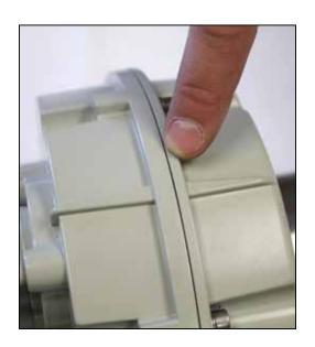
18. Now it is important to note the placement of the lead transducer. There are two markings that are used to identify the lead transducer, one is on the widest part of the transducer body in the form of a raised line, and the other is a notch just above the threads on the neck of the transducer.
