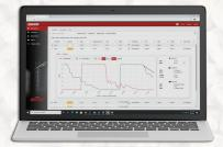
A chart showing sensor level readings converted to tons overlays the ADFI slope indicating consumption and filling, generated for a specific date range. Charts can be created based on other reading types including delivery capacity, distance, percent full, and sensor battery life. Drilling down further, the most recent sensor reading is timestamped, with reporting on all bin parameters.
