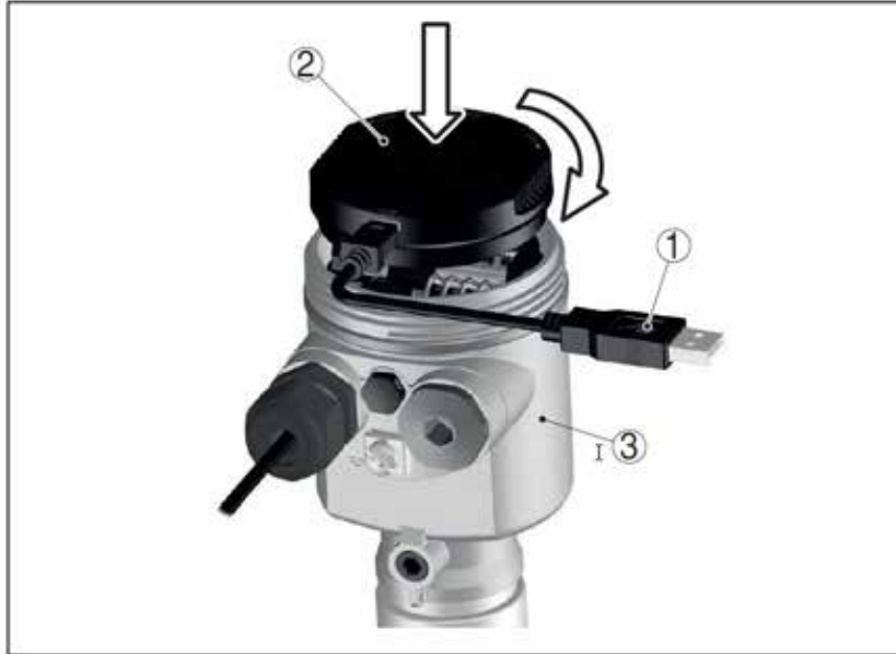
Fig. 45: Connection of the PC directly to the sensor via the interface adapter
