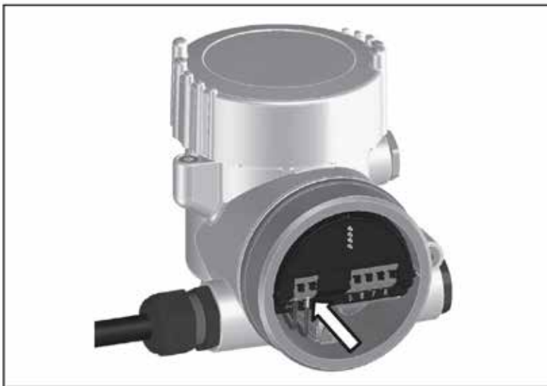
Fig. 27: Connection steps 5 and 6 - Double chamber housing
