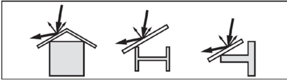
Fig. 18: Cover flat, large-area profiles with deflectors
