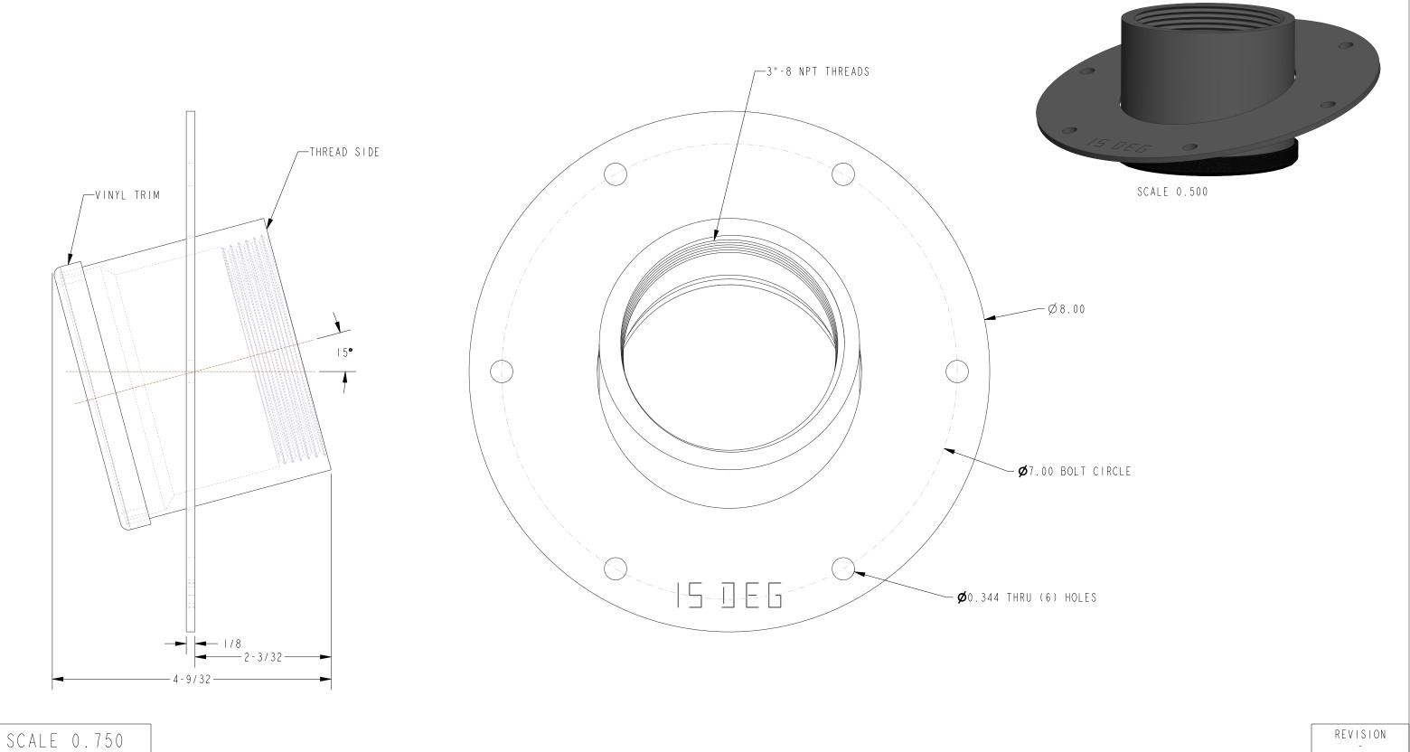
PAGE I OF I TITLE: MTG. DIM, MOUNTING PLATE, SBMP-15 Model No.: SBMP-15 P/N: 416-0397 DWG No.: 418-0273 MATERIAL: BLK POWDER COATED STEEL
